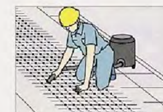
3. Clean up the dust on the ground
